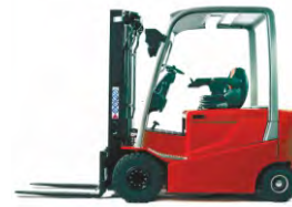
Elektro-4-Radstapler 2,0 - 5,0 to 80 Volt
