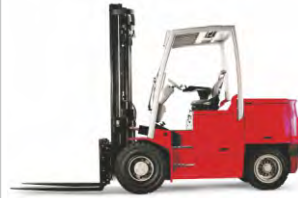
Elektro-4-Radstapler 6,0 - 8,5 to 80 Volt
